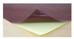
FIBERLAM RR15AD is glass fabric coated with PTFE (Teflon), both side laminated with cast PTFE multilayer film then one side coated with high temperature resistant, silicone pressure sensitive adhesive.
